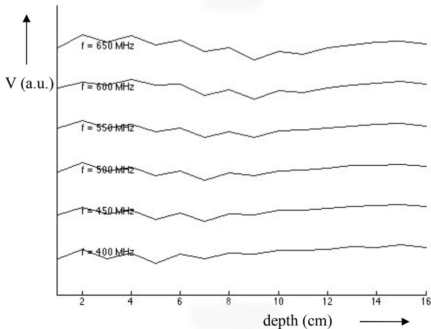
**Fig. 3:** Voltages in arbitrary units measured in air at the outputs of the detectors in function of the frequency and of the depth (the curves have been shifted on y axis for clarity)
