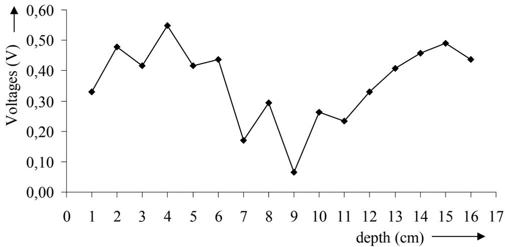
**Fig. 4:** Standing wave measured at 600 MHz in air
