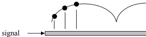
**Fig. 1:** spatial sampling (points) of the standing wave (in dark) occurring in an open circuited waveguide (in grey)
