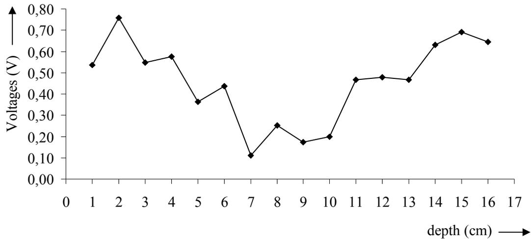
**Fig. 6:** Standing wave measured at 150 MHz in methanol
