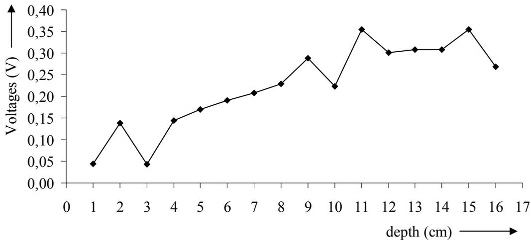
**Fig. 7:** Standing wave measured at 100 MHz in 1-butanol
