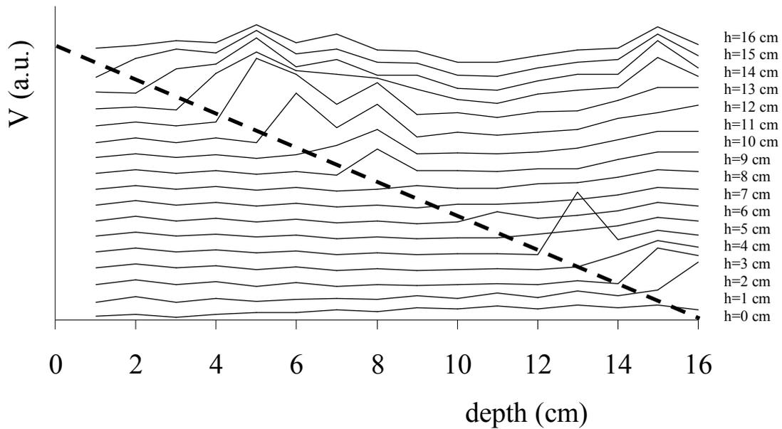
**Fig. 8:** Voltages (in arbitrary units) measured at 200 MHz in a mixing of glass marbles progressively filled with distilled water (the curves have been shifted on y axis for clarity).
