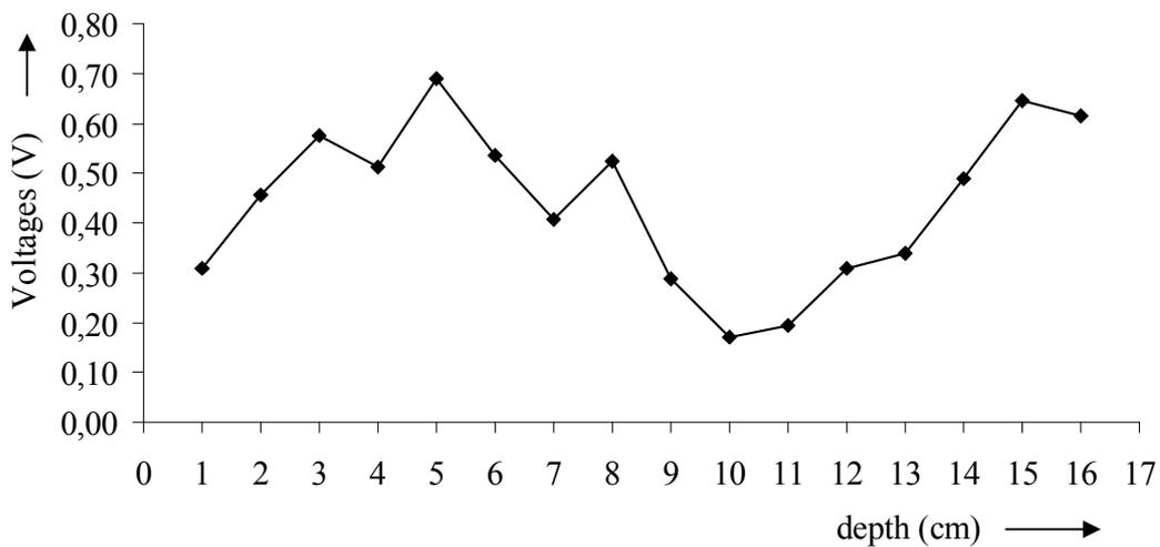
**Fig. 5:** Standing wave measured at 150 MHz in distilled water
