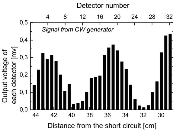
Fig. 6. DC voltage measured on the 32 power detectors placed along the standing wave.
