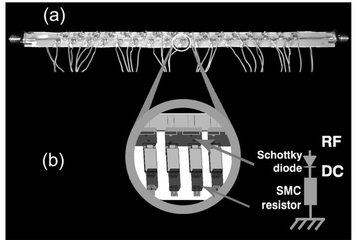
Fig. 3. (a) Photograph of the full spectrometer built with 32 unit cells. (b) 3D view (zoom) and diagram showing details of the cell (diode and resistor).
