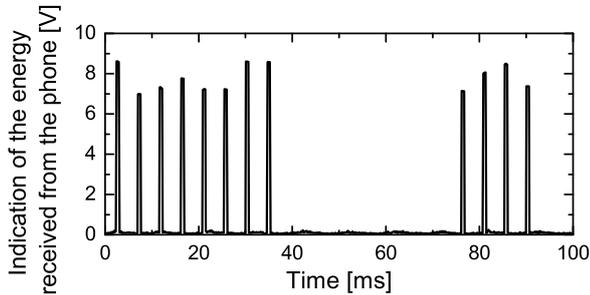
Fig. 8 Measurement of the temporal spikes emitted by a cell phone
