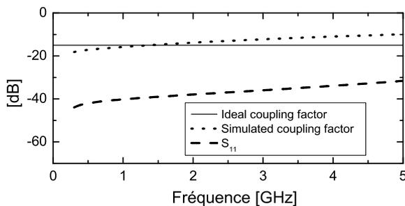
Fig. 2. Reflection coefficient S11 of the unit cell (dashed line) and energy coupled from the microstrip to the detector (dotted line). The maximum of efficiency is obtained at -15dB (solid line).
