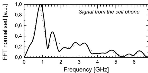
Fig. 10. FFT of the standing wave shown in fig. 8 with interpolation (solid line) and without interpolation (dotted line)
