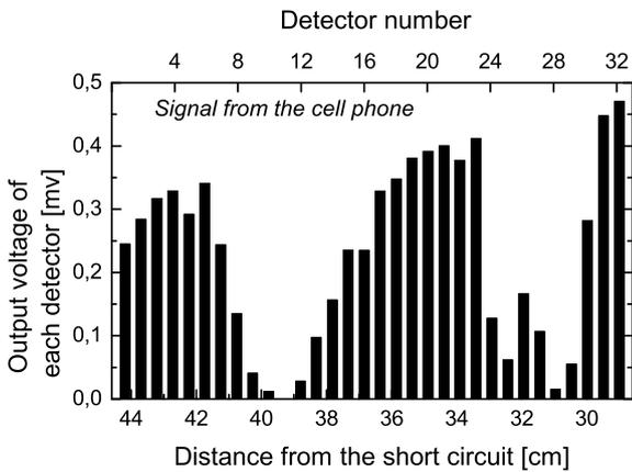
Fig 9 Standing wave corresponding to the first spike shown in Fig 8
