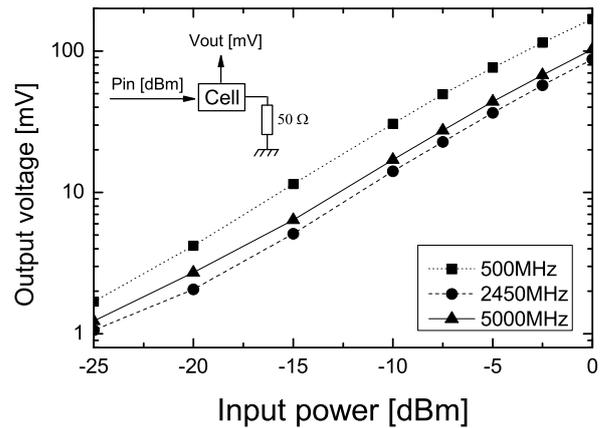
Fig. 4. Detected voltage versus input power in a single detector at 500 MHz (dotted line), 2450 MHz (dashed line) and 5 GHz (solid line).
