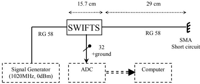
Fig. 5. Measurement setup for RF interferometry using the SWIFTS.
