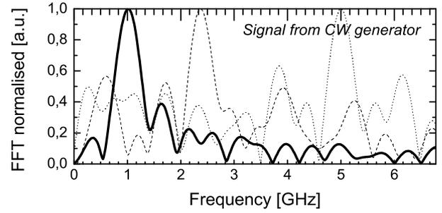
Fig. 7. Fast Fourier Transform (FFT) of the 1 GHz standing wave shown in Fig. 6 (bold line) together with similar results at 2.45 GHz (dashed line) and 5 GHz (dotted lines).
