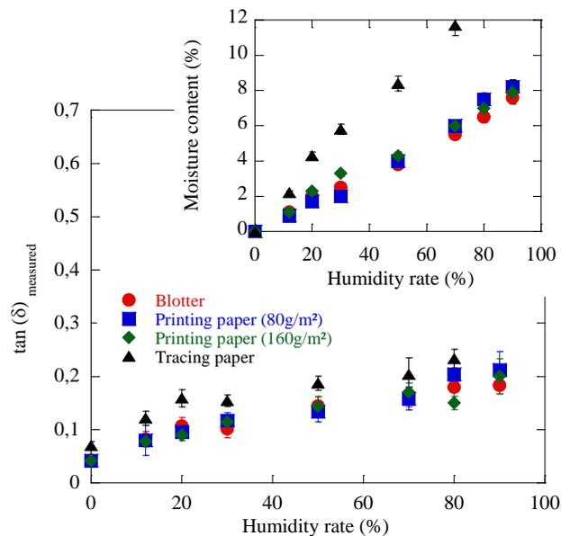
Fig. 1. Losses of the four papers at 900 MHz with the humidity rate of atmosphere. Inset : Moisture content of papers with the humidity rate.
