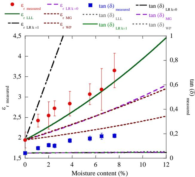
Fig. 3. Dielectric real permittivity and losses of Blotter at 900 MHz with free water properties compared to the simulation of LLL, LR for  $k=1$ , LR for  $k=0$ , MG and Wiener for perpendicular orientation of molecules.
