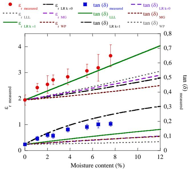
Fig.4. Dielectric real permittivity and losses of Blotter at 900 MHz with bound water properties compared to the simulation of LLL, LR for  $k=1$ , LR for  $k=0$ , MG and Wiener for perpendicular orientation of molecules.
