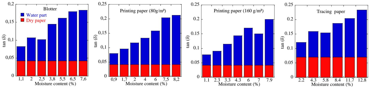
Fig. 2. Contribution of the water (blue) and the dry paper (red) to the losses at 900 MHz.
