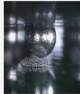
Figure 1. The BGA package has not been placed into the paste deposit.
