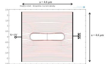
Figure 4. Current streamlines, longitudinal excitation@  $f = 1\text{MHz}$
