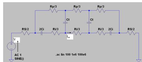
Figure 3. Equivalent circuit of the box, longitudinal Excitation
