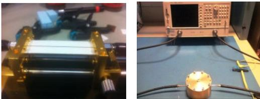
The complex permittivity is determined by resonant cavity method at 2.45GHz → This method can be only performed on a given frequency.
