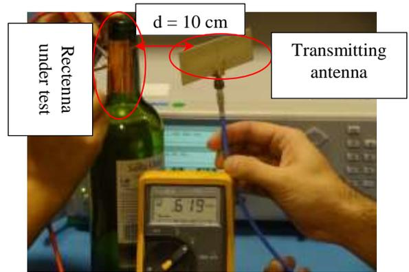
Fig. 9. Photograph of measurement process.
