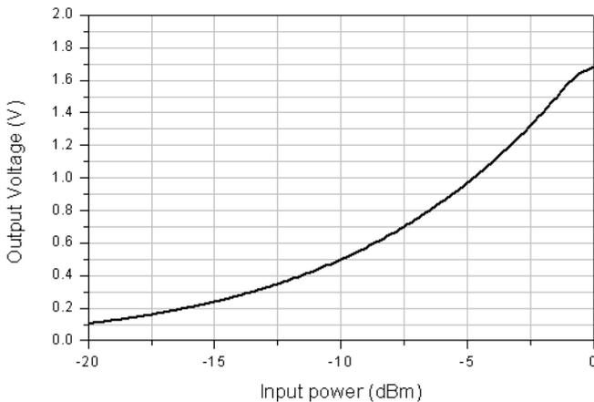
Fig. 8. DC voltage of the rectifier circuit depending on input power.
