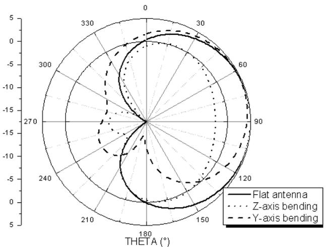
Fig. 6. Far-field radiation pattern of flat and bended antennas.
