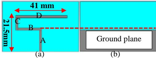
Fig. 2. Antenna structure simulated under CST a) Top view b) Bottom view. A, B, C and D allows the identification of each section of the antenna.
