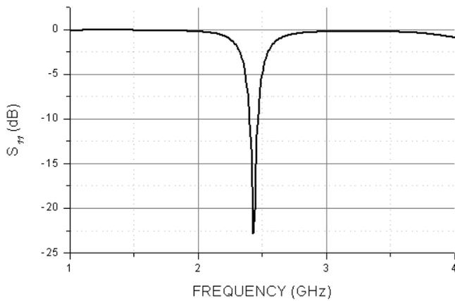
Fig. 3. Reflection coefficient of the monopole antenna simulated under CST.
