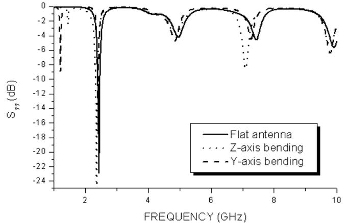
Fig. 5.  $S_{11}$  parameters of flat and bended antennas.
